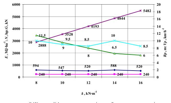
$- G, kN \rightarrow N, hp \rightarrow E, MJ \cdot ha^{-1} \rightarrow Bp, m \rightarrow Vp, km \cdot h^{-1}$ Fig. 4. Depending on the total energy costs, parameters and modes of operation of the unit on the specific resistance of the soil snarl
