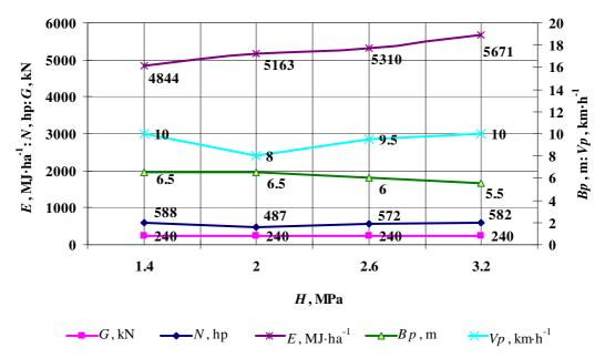
Fig. 5. Depending on the total energy costs, parameters and modes of operation of the unit on the hardness of the soil
