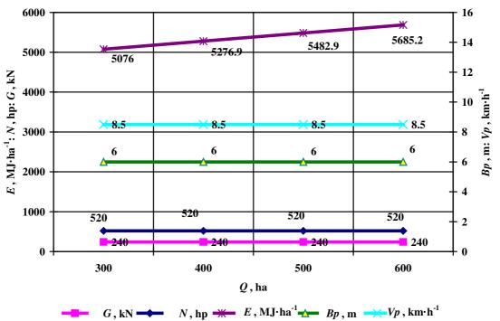
Fig. 3. Depending on the total energy costs, parameters and modes of operation of the unit on the annual load of the snarl
